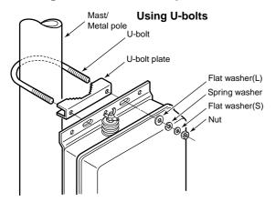
**WARNING:** Mount the AT-140 securely with the supplied nuts and bolts. Otherwise, vibrations and shocks due to waves, etc. could loosen the antenna tuner making if fall, causing personal injury.
