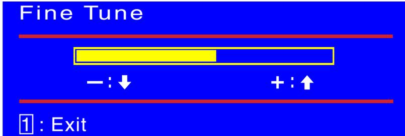
**Fine Tune:** To adjust the delay time.
