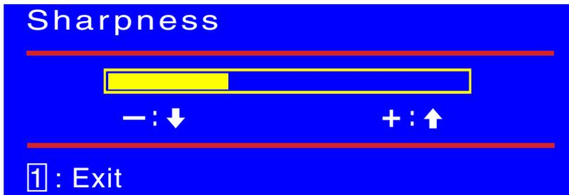
**Sharpness:** Adjusts the clarity of a non-SXGA (1280x1024) signal.
