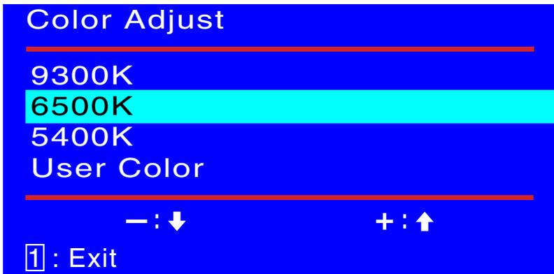
**Color Adjust:** Provides four preset color adjustments:
