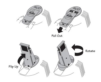
ON/OFF SWITCH FOR RCD H AND HR
