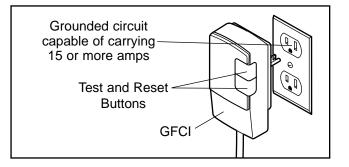
ning, press the GFCI "test" button. The spa should shut off. Press the "reset" button. The spa should resume normal operation. If the spa continues to run after the "test" button is pressed, then the GFCI is damaged. Do not use the spa until the GFCI has been repaired or replaced by a qualified electrician.
