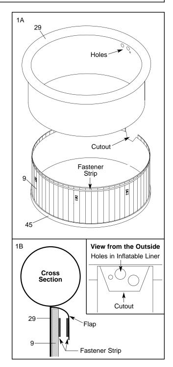
2. Orient the dry side jet pack (A) as shown and place it near the three holes in the Inflatable Liner (29).
