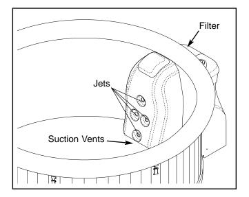
The suction vents, located on the bottom side of the wet side jet pack, pull the water into the spa unit in order to operate the system. The suction covers should always be in place over the suction vent. Never operate the spa without the suction covers in place.
