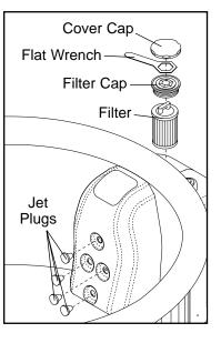
insert the filter and fill the filter housing to the top with water. Replace and hand tighten the filter cap; then, use the included flat wrench to tighten the filter cap an additional 1/4 turn. Press the cover cap back onto the filter cap. Remove the jet plugs and store them in the pouch inside the cover. **IMPORTANT: The spa jet unit may be seriously damaged if the water pump is not properly primed or if the filter cap is not re-attached and fully tightened.**
