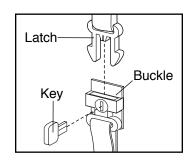
unlock the buckles, insert the key and turn it counterclockwise a quarter turn.
