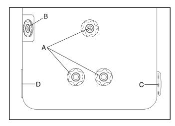
The **whirlpool jet** (B), located on the left side of the spa jet unit, directs the flow of the water to create a whirlpool action in the hydrotherapy spa.
