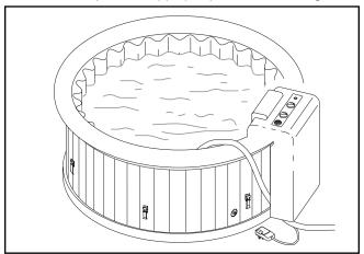
hose to siphon the water. Place one end of the hose in the spa and hold it in front of a hydrotherapy jet until there is a flow of water coming out of the hose. Turn off the spa unit and unplug the power cord. The unit will be damaged if it is run without water circulating. Be sure the end of the hose in the spa is on the floor of the spa.
