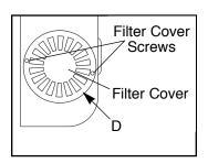
ment by removing the filter cover and the two filter cover screws and then pulling the filter from the spa jet unit.
