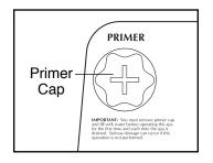
unit may be seriously damaged if the pump is not properly primed, or if the primer cap is not replaced and fully tightened.
