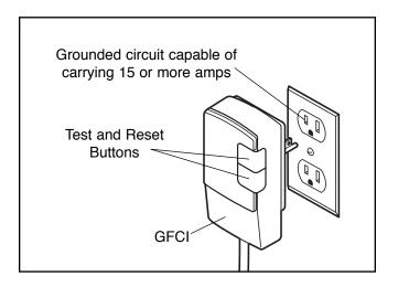
When connecting the power cord, plug the power cord directly into a grounded circuit capable of carrying 15 or more amps. No other appliance should be on the same circuit. Replace the power cord immediately if it becomes damaged.
