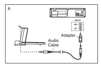
B. Plug one end of the audio cable into the jack beneath the console. Plug the other end of the cable into the included adapter. Plug the adapter into an RCA Y-adapter (available at electronics stores). Next, remove the wire that is currently plugged into the AUDIO OUT jack on your VCR and plug the wire into the unused side of the Y-adapter. Plug the Y-adapter into the AUDIO OUT jack on your VCR.
