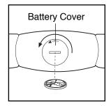
Remove the old battery from the sensor unit. Insert a new **CR 2032 battery**, making sure that the writing is on top. In addition, make sure that the rubber gasket is in place in the sensor unit. Replace the battery cover and turn it to the closed position.
