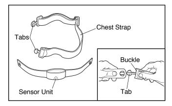
Next, wrap the heart rate monitor around your chest and attach the other end of the chest strap to the sensor unit. Adjust the length of the chest strap, if necessary. The heart rate moni-
