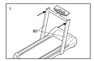
Cut any plastic ties from the Right and Left Handrails (93, 94). Set the Right Handrail (the longer Handrail) on the right Upright (80). Finger tighten a Short Handrail Bolt (59) with one of the two metal Handrail Washer (95) into the Upright and the Right Handrail. Do not tighten the Handrail Bolt yet.
