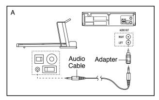
B. Plug one end of the audio cable into the jack on the front of the treadmill near the power cord. Plug the other end of the cable into the included adapter. Plug the adapter into an RCA adapter (available at electronics stores). Next, remove the wire that is currently plugged into the AUDIO OUT jack on your VCR and plug the wire into the unused side of the RCA adapter. Plug the RCA adapter into the AUDIO OUT jack on your VCR.
