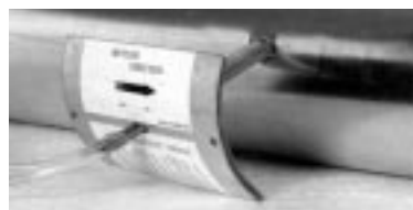
figure 11.3 Inserting Air flow grid in duct
