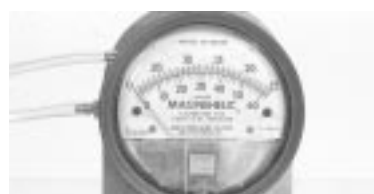
figure 11.3 Magnehelic Gauge at «0»
