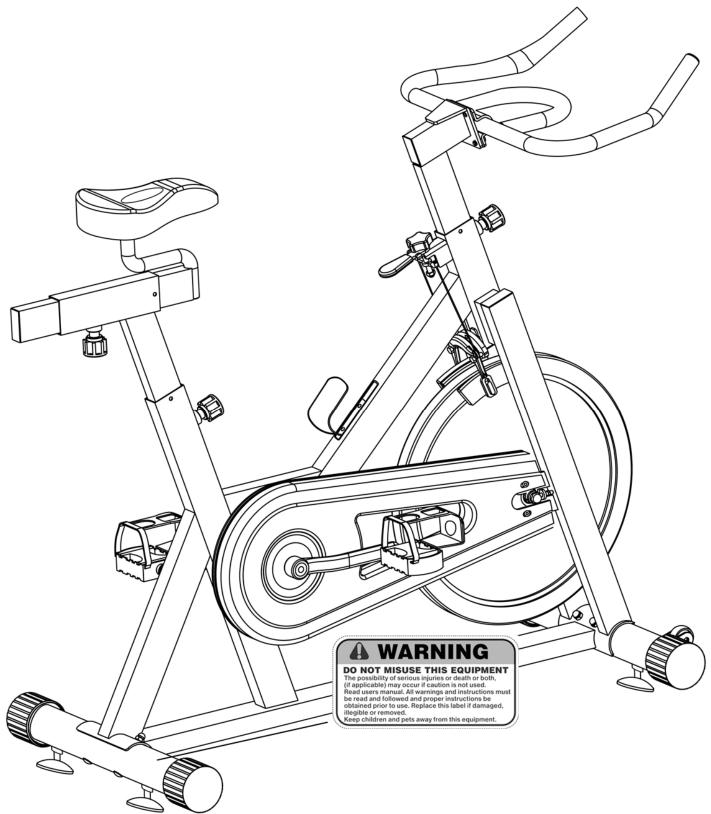
The Warning Labels and Caution Label shown here have been placed on the Rear Stabilizer, Main Frame. If the labels are missing or illegible, please call customer service at 1-800-999-8899 for replacement. Apply the labels in location shown.
