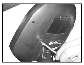
**STEP 14:**Securely tighten the *COMPUTER (#8)* with four computer fix screws and spring washers.
