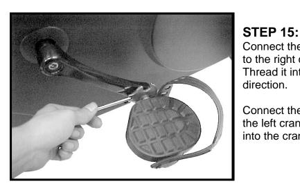
Connect the **RIGHT PEDAL** (#13) (marked "R") to the right crank of **MAIN FRAME** (#1). Thread it into the crank in the clockwise direction.
