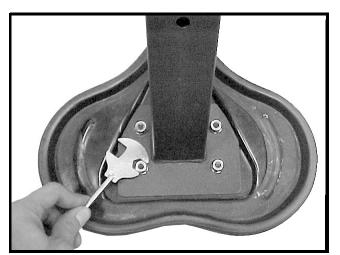
STEP 8: Attach the SEAT POST #(5) to the SEAT #(6). Securely tighten with SPRING WASHERS and NYLON NUTS.
