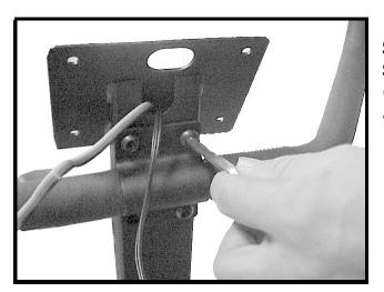
STEP 11: Securely tighten the *HANDLE BAR (#9)* to *COMPUTER POST (#4)* with four *ALLEN KEY BOLTS (C)*.
