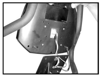
STEP 13: Attach COMPUTER (#8) onto COMPUTER POST (#4). Connect the COMPUTER WIRE (#7), SENSOR WIRE (#14) and HAND PULSE SENSOR to the back of COMPUTER (#8).
