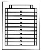
Slide weight plates onto Guide Rod from top to bottom.
