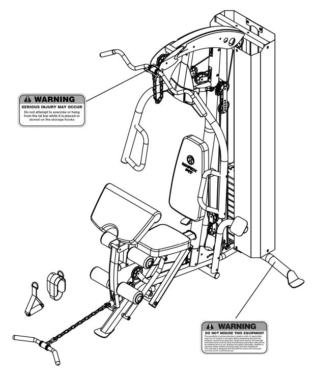
The warning labels shown here have been placed on the Rear Base and Upper Frame. If the labels are missing or illegible, please call customer service at 1-800-888-8899 for replacements. Apply the labels in the location shown.
