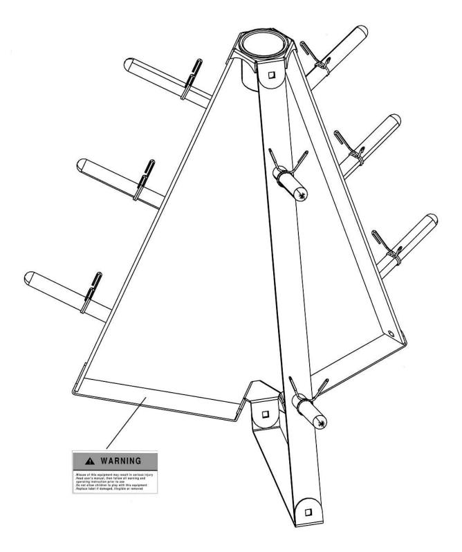
The Warning Label shown here has been placed on the Base Frame. If the label is missing or illegible, please call customer service at 1-800-999-8899 for replacement. Apply the label in location shown.
