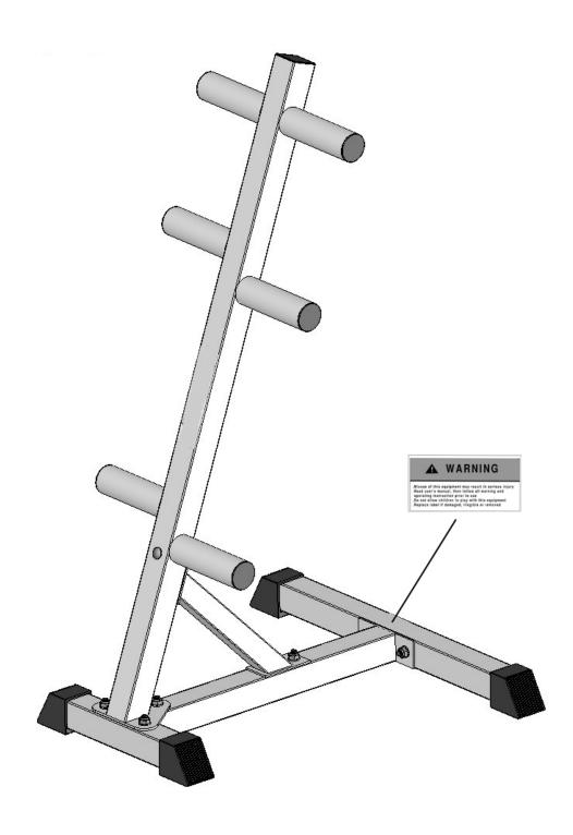
The Warning Label shown here has been placed on the base of Rear Stabilizer. If the label is missing or illegible, please call customer service at 1-800-999-8899 for replacement. Apply the label in location shown.
