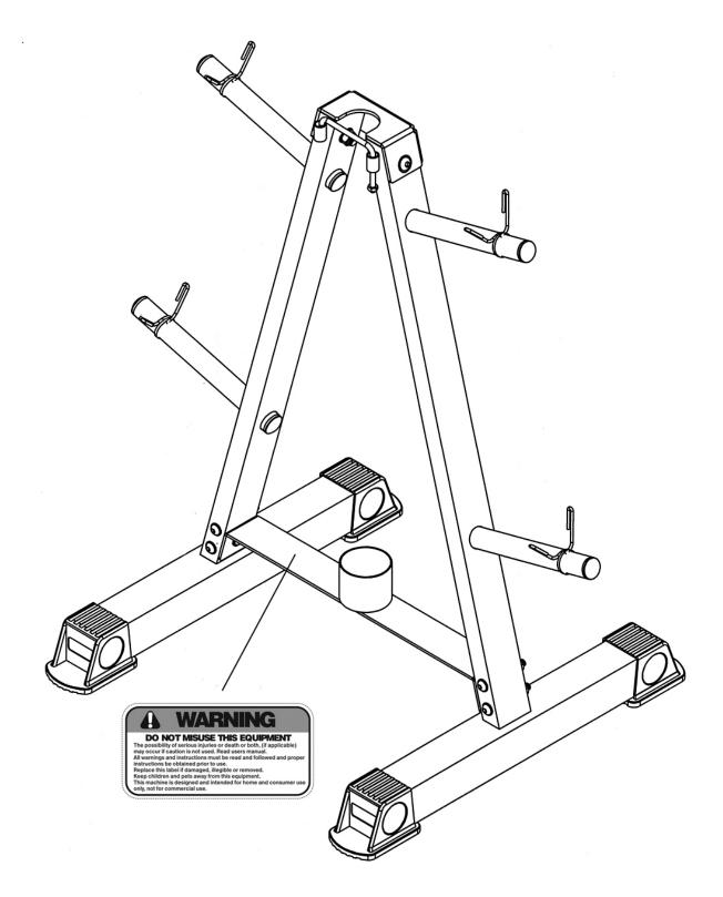
The warning labels shown here have been placed on the Cross Brace. If the labels are missing or illegible, please call customer service at 1-800-888-8899 for replacements. Apply the labels in the location shown.
