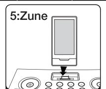
Insert a Zune into the dock with proper insert (Zune must not be in a skin or case). The Zune will charge while docked. Press the III Button on the ZN90 to play your Zune.
