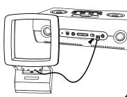
Snap AM antenna into stand, then plug antenna cable into socket on back of ZN90. Move antenna 12" away.
