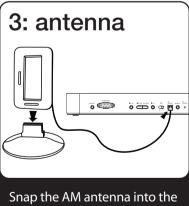
provided stand, then plug the antenna cable into the socket on the back of the iH51. Move the antenna 12" away.
