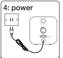
Plug the AC cable on the back of the iH51 subwoofer into a working wall socket
