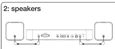
Attach a speaker cable from the right speaker (R speaker) and left speaker (L speaker) jacks on the back of the receiver to the jack on the back of each matching speaker.
