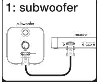
Connect the provided connector cable from the back of the subwoofer to the back of the receiver and tighten screws.
