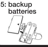
Remove the battery compartment door on the bottom of the receiver and insert 2 AA batteries (match + and - polarity to diagram in compartment). Replace door.
