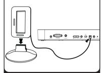
Snap the AM antenna into the provided stand, then plug the antenna cable into the socket on the back of the iP51. Move the antenna 12" away.
