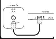
Connect the provided connector cable from the back of the subwoofer to the back of the receiver and tighten screws.
