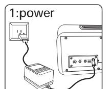
Attach AC adaptor plug to jack on back of the unit and plug the other end into a wall socket.
