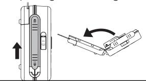
To open the unit, use thumb to push the two sliding lock bars on either side UP to unlatch. To close cover, push lock bars back down.
