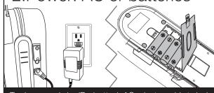
To charge and play iPod, attach AC adaptor cable to jack on left of the iH20 (under rubber tab) and plug the other end into a working AC outlet. Does not charge batteries. For portable operation (in shower, etc.), open the battery door located inside the unit above the iPod dock. Install 4 AA batteries (match + and - polarity in diagram).
