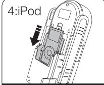
Insert iPod into dock with proper insert. Once iPod is docked, close the iH20. When running on AC power, the iPod will charge while docked. Press the Play Button on the iH20 to play your iPod.
