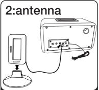
Snap AM antenna into provided stand, then plug antenna cable into socket on back of unit. Move antenna 12" away.
