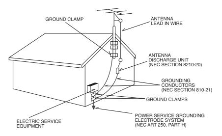
9 Power Lines - An outside antenna system should not be located in the vicinity of overhead power lines or other electric light or power circuits, or where it can fall into such power lines or circuits. When installing an outside antenna system, extreme care should be taken to keep from touching such power lines or circuits as contact with them might be fatal.
