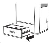
Press on the dock door on the front of the unit to release the universal dock. Push dock back into unit when not in use.
