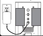
Attach AC adaptor cable to the DC jack on back of the iP39 and plug the other end into a working wall socket to play and charge iPhone/iPod and to provide power to the USB port
