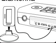
Snap AM antenna into provided stand, then plug antenna cable into socket on back of iP99. Move antenna 12" away.
