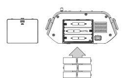
The unit can also be powered by batteries. (Requires 6 C size batteries, not included.
