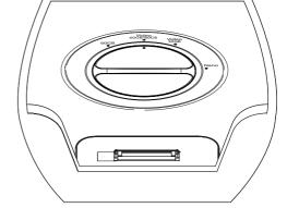
•The 30-pin connection for an iPod slides to the left for iPod nanos, or to the right for all other iPod models.
