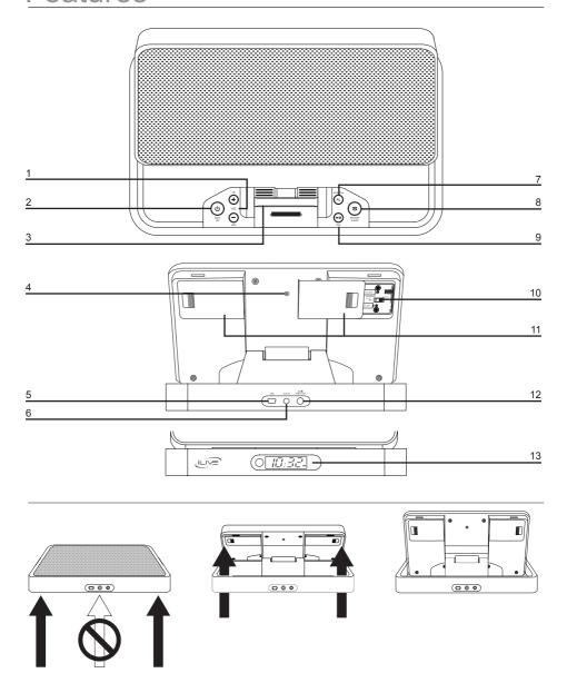
When un-folding the player, press up on the back corners and not the center. Opening incorrectly and with too much force could damage the player.
