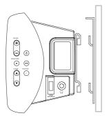
Hanging the wall mount is as easy as screwing the two included brackets into the wall and hanging the player on them. It is recommended that you use 3 screws to secure each individual bracket to the wall.
