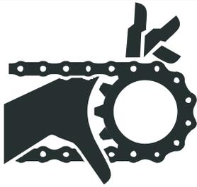
Moving parts can crush and cut. Keep hands clear. Do not operate without guards in place. Failure to do so could result in serious injury.
