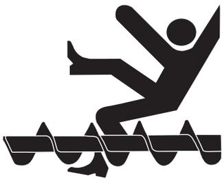
Rotating auger will crush and cut. Auto equipment can start at anytime. Do not enter until electric power is locked in off position. Failure to do so will result in serious injury or death.
