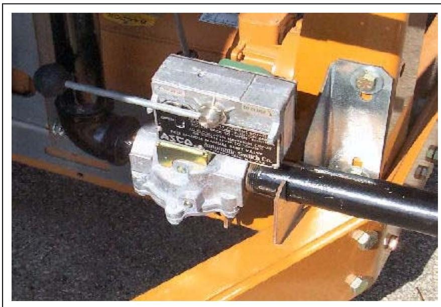
Figure 5A Asco Safety Shut Off Valve
