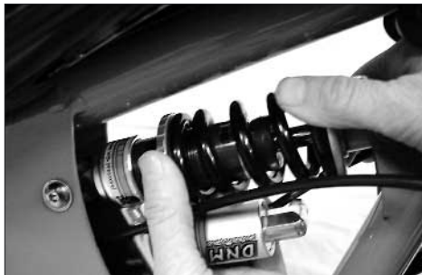
Turn the knurled ring to adjust the pre-load.
