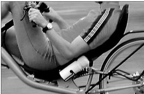
An ideal position for water bottle cages is at the side of the seat.
