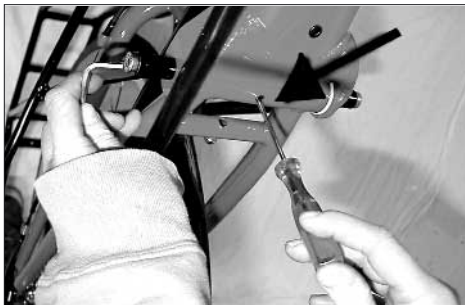
You can prevent the axle from turning by inserting a thin metal rod in the hole of the axle.
