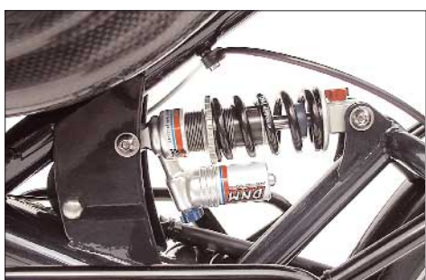
Suspension element ST8ARC with adjustable damping and piggy-back gas tank.
