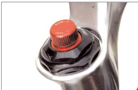
Turning knob for the adjustment of the damping of the suspension fork MEKS Carbon AC.
