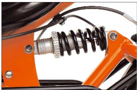
Suspension element DV-22 with fixed damping rate.
