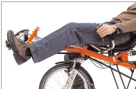
Adjust the front boom so that your knee will not be fully straightened when pedaling.
