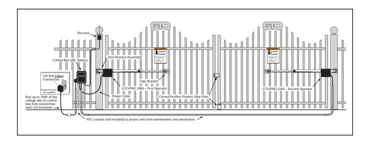
The open position stop for the second gate is installed the same as the first gate. See instructions on page 16.
