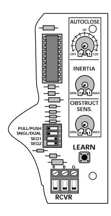
**AUTO CLOSE** (auto close timer): Determines how long the gate will remain open before it automatically closes. The limits are **OFF** to 120 seconds. The factory setting is **OFF**.
