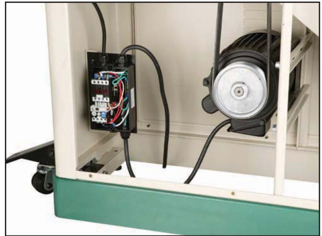
Figure 78. Magnetic switch wiring.
