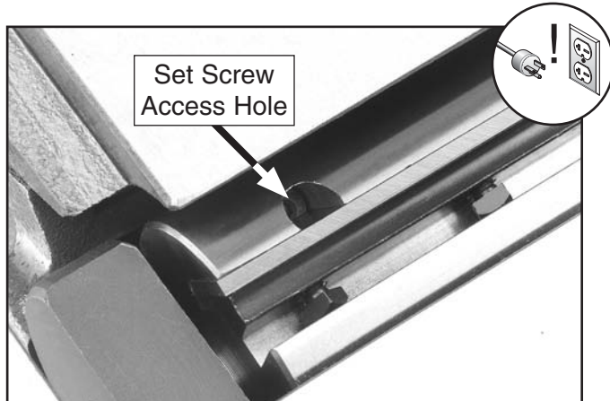
Figure 57. Set screw access hole.
