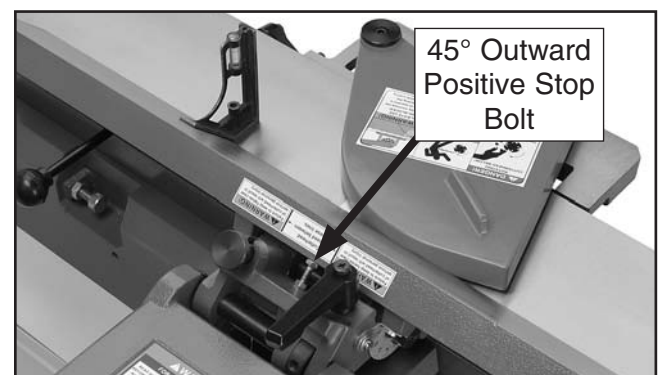
Figure 76. Adjusting fence 45° outward.
