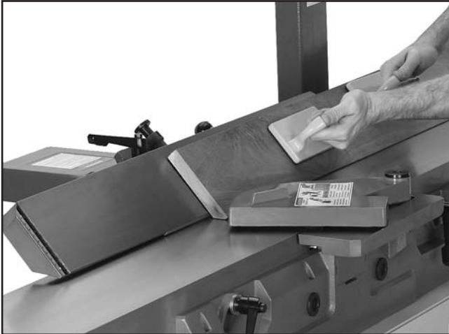
Figure 41. Fence setup for a bevel cut of 45°.
