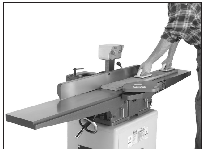
Figure 26. Typical surface planing operation.
