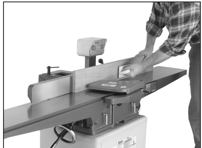
Figure 28. Typical edge jointing operation.
