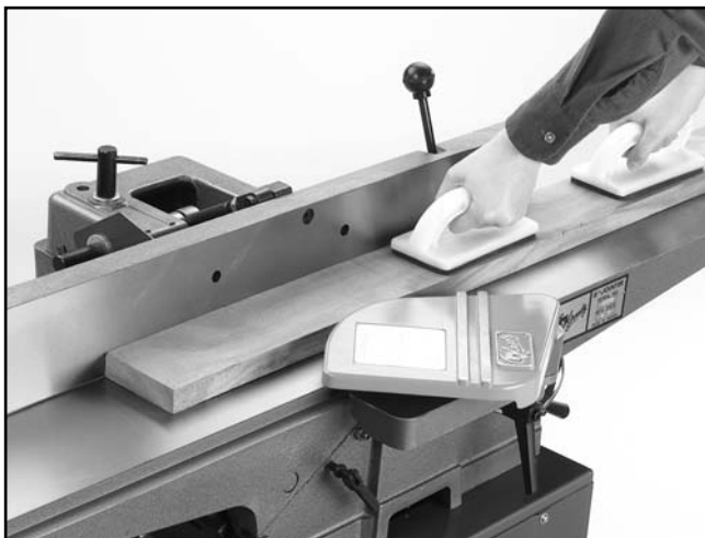
Figure 27. Correct method for surface planing.
