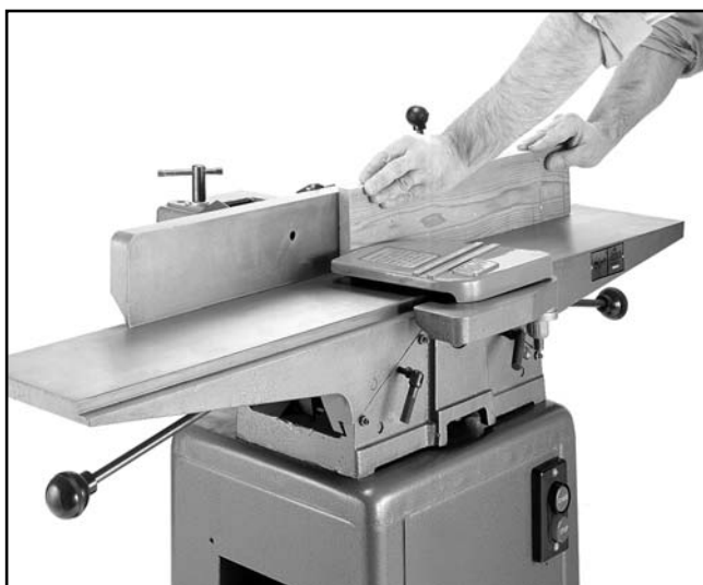
Figure 25. Operator position for edge jointing.
