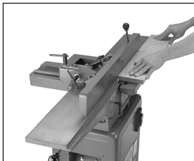
Figure 28. Correct operator position for rabbet cutting.
