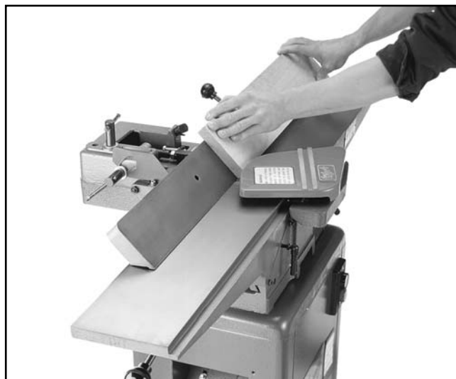
Figure 26. Fence position for bevel jointing.
