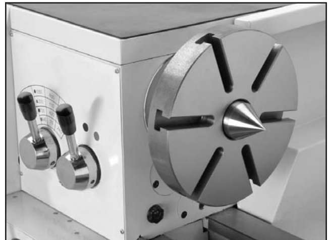
Figure 25. Faceplate and dead center setup.
