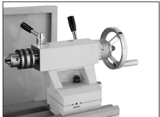
Figure 18. Setting up tailstock for drilling.
