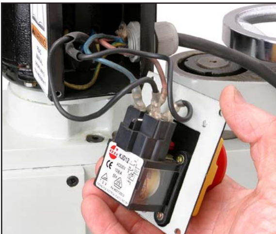
Figure 66. Mill power switch.
