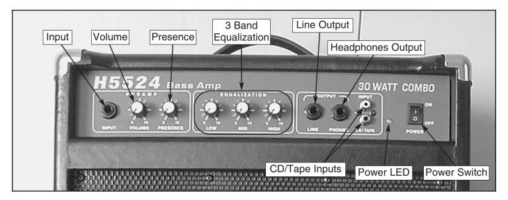
**INPUT**—Connect your guitar here, using a shielded instrument cable with a ½" jack.
