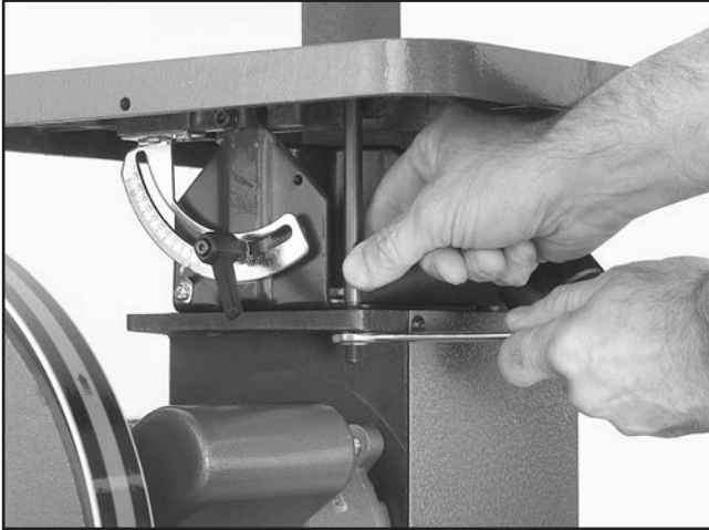
Figure 11. Squaring the sanding table.
