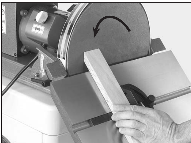
Figure 18. Disc sanding with table tilted.
