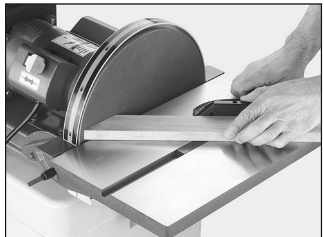
Figure 19. Disc sanding with miter.
