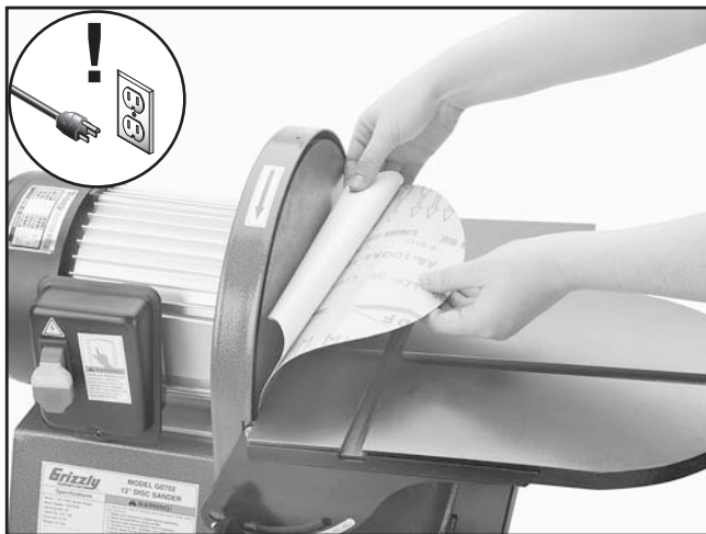
Figure 7. Sandpaper being slipped between the disc and table.
