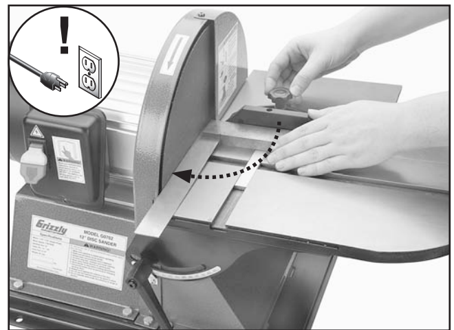
Figure 18. Squaring miter gauge to disc.
