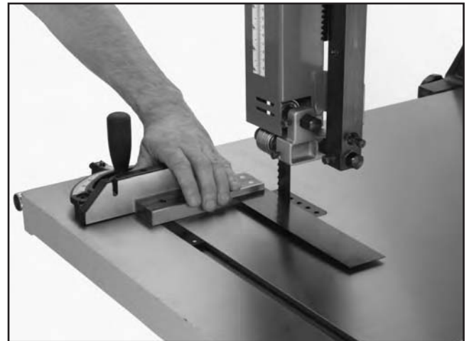
Figure 17. Squaring miter gauge to blade.
