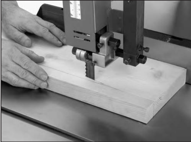
Figure 35. Blade leading away from line of cut.
