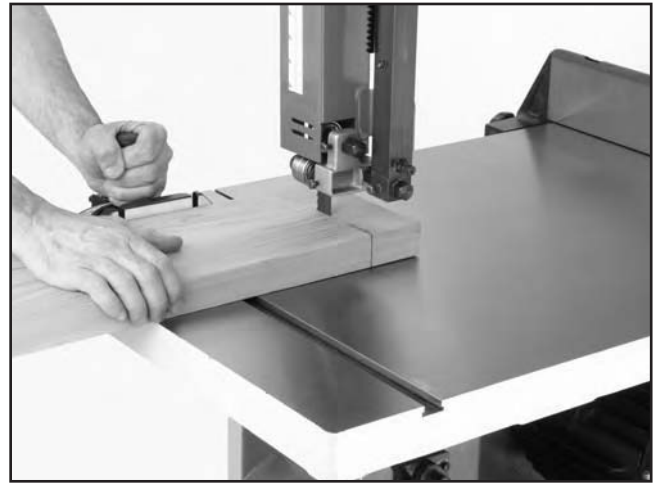
Figure 32. Crosscutting with the miter gauge.
