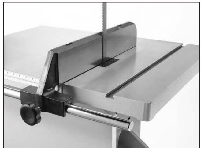
Figure 19. Fence flush with blade.
