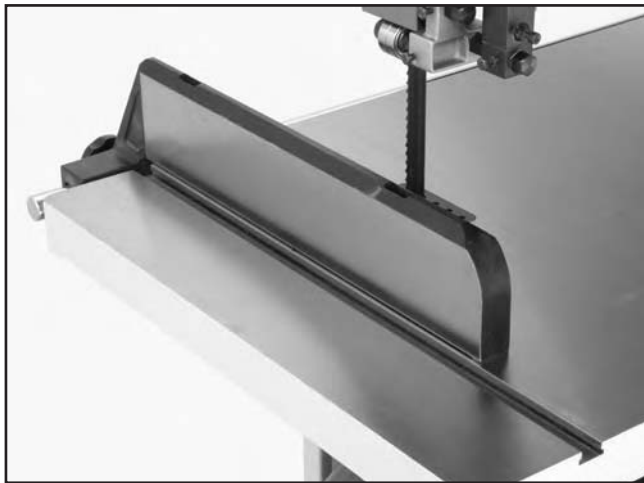
Figure 18. Fence square with miter slot.
