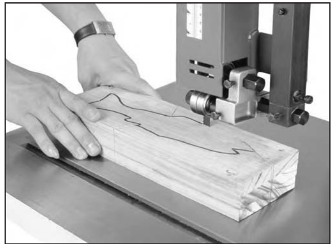
Figure 36. Cutting multiple pieces at once.
