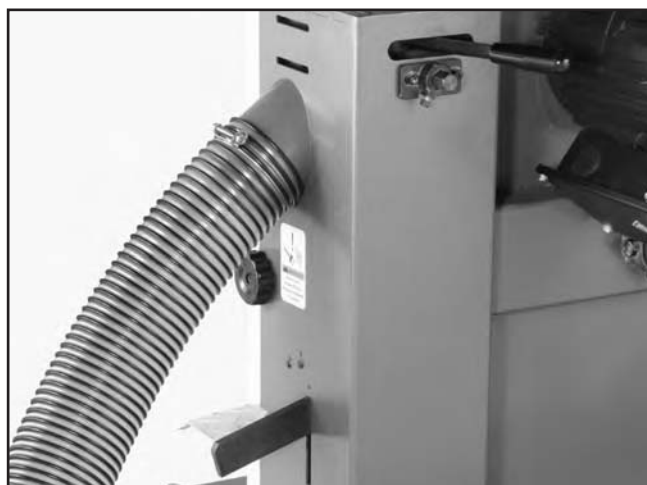
Figure 20. Dust hose attached to dust port.
