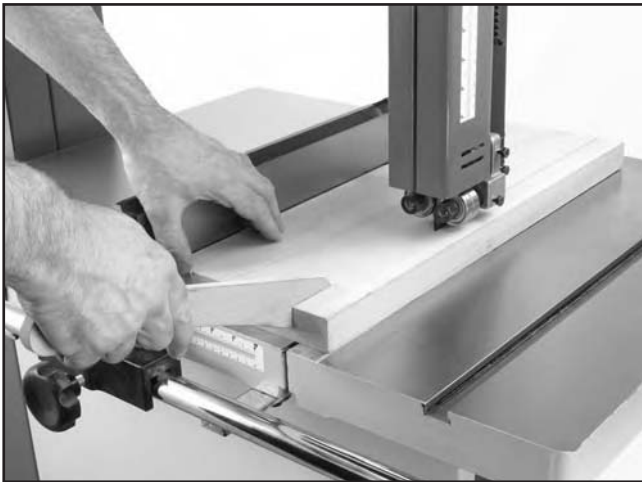
Figure 31. Ripping with a push stick.
