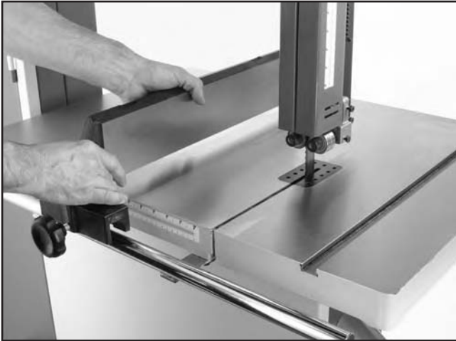
Figure 11. Installing fence onto rail.
