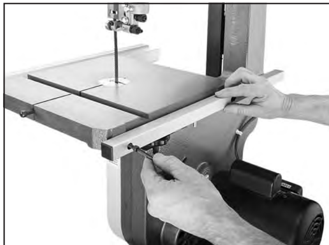
Figure 19. Attaching the rear fence rail.
