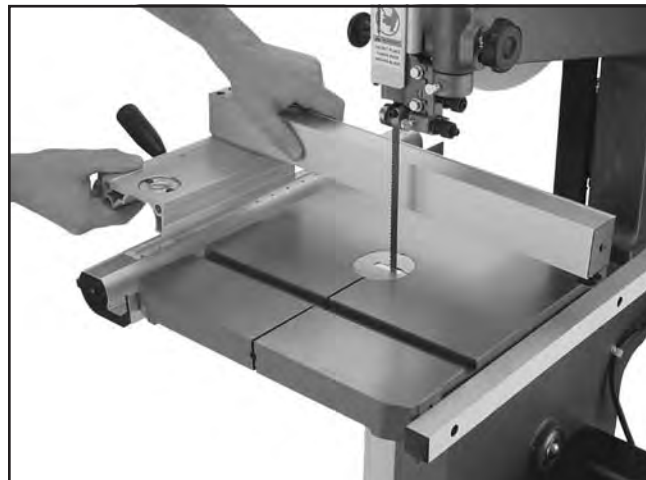
Figure 20. Placing the fence onto the rails.
