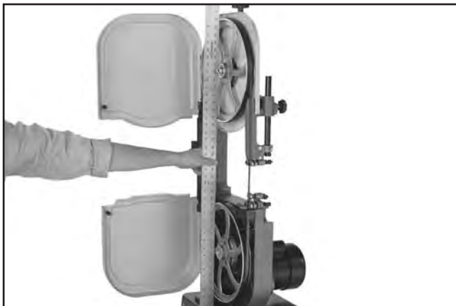
Figure 62. Checking if the wheels are coplanar.
