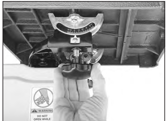
Figure 17. Securing table to the trunnion.
