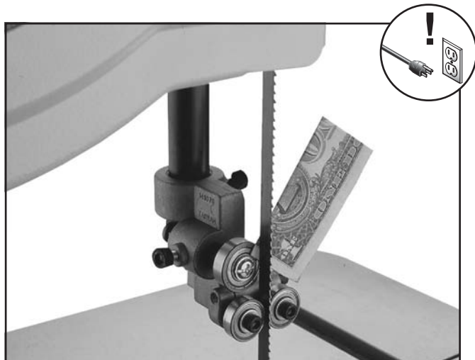
Figure 32. Dollar bill folded twice to make a quick 0.016" gauge.
