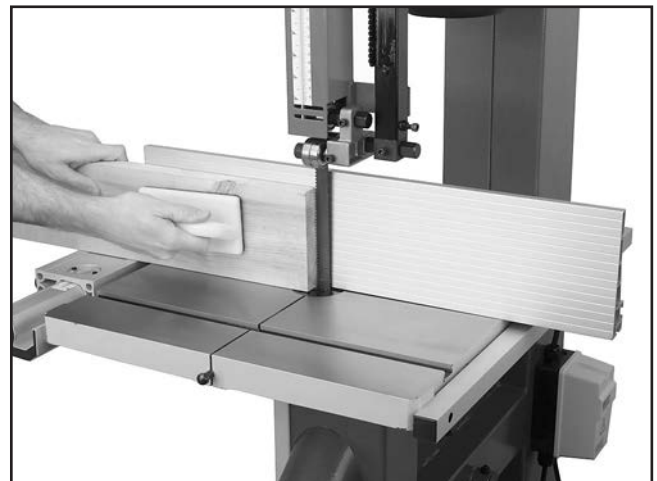
Figure 33. Typical resawing operation.
