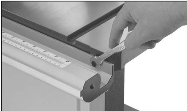
Figure 13. Fastening front fence rail to table.
