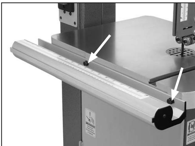
Figure 17. Installed front rail.
