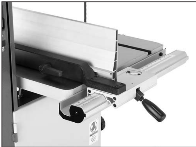
Figure 20. Correctly installed fence.
