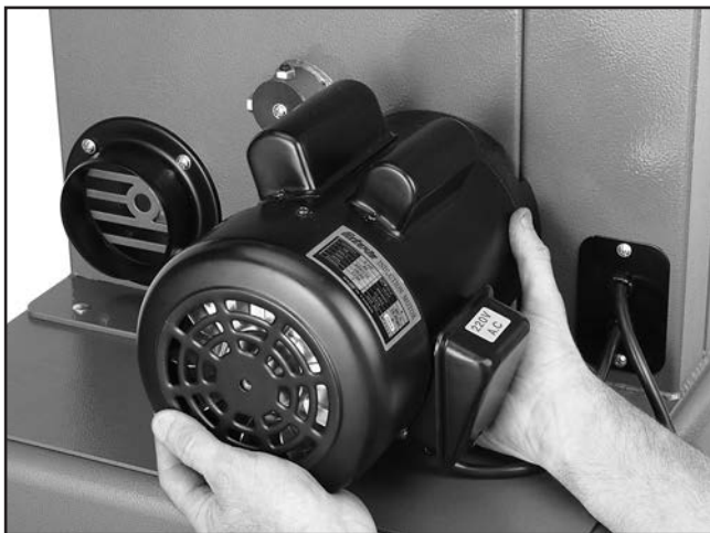
Figure 13. Installing motor (outside view).
