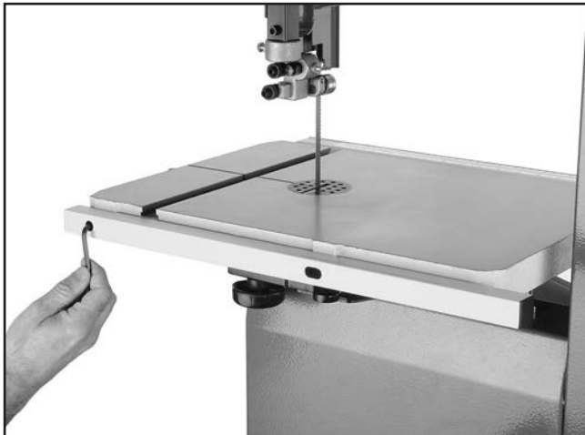
Figure 16. Rear rail installed.
