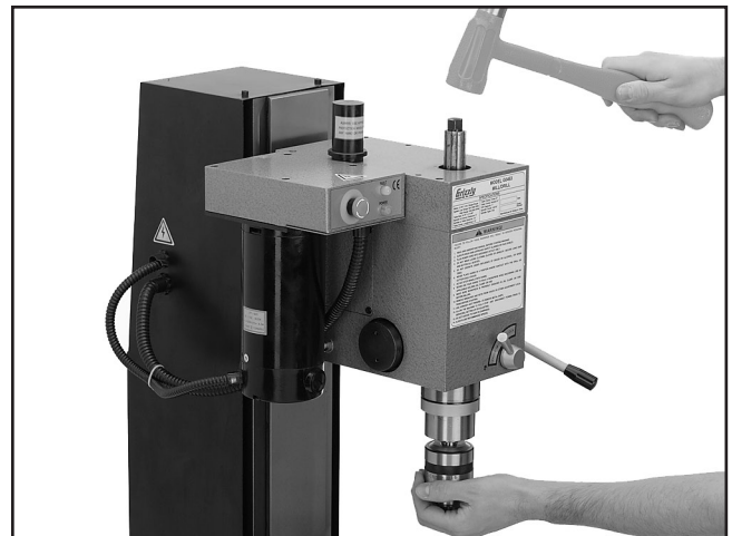
Figure 9. Striking the drawbar.
