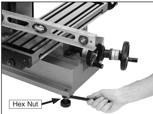
Figure 6. Leveling the mill/drill.
