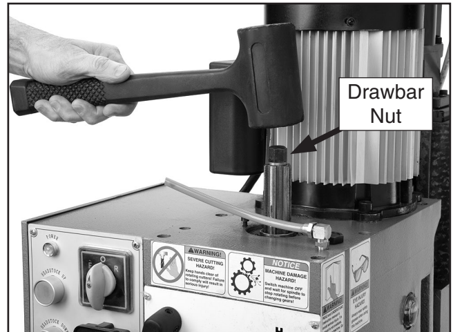
Figure 14. Unseating the arbor/cutter.
