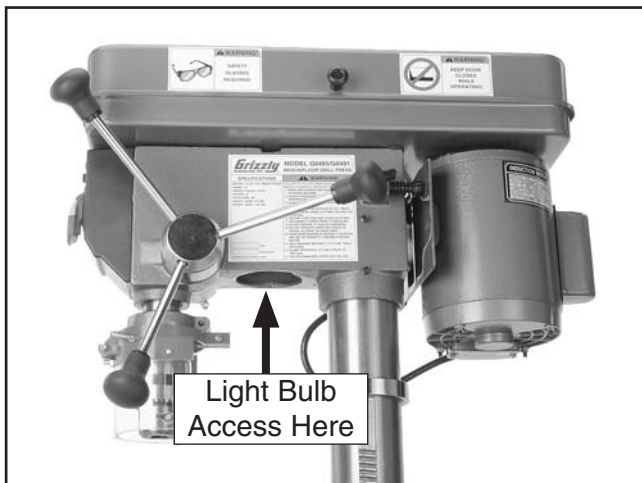
Figure 20. Light bulb access location.
