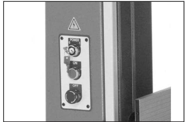
Figure 38. G0514X switch disabling key and ON/OFF switch.
