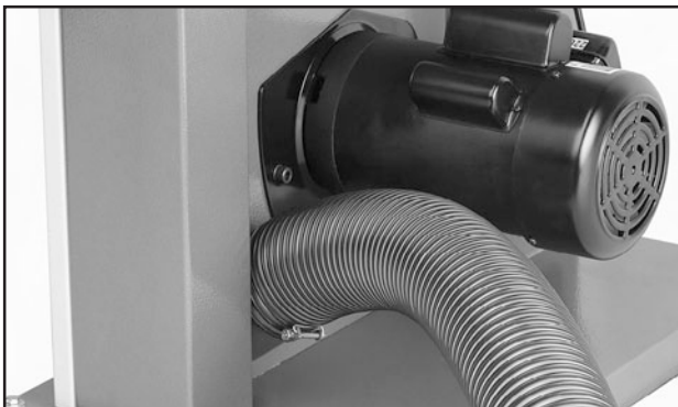
Figure 31. Dust hose attached to one of the two dust ports.
