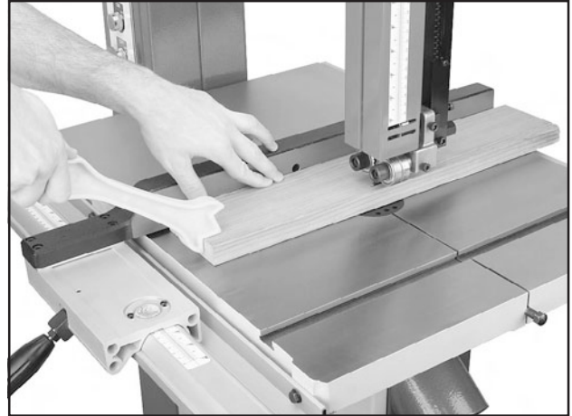
Figure 62. Ripping with a push stick.
