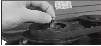
Figure 25. Tightening nut on drawbar.
