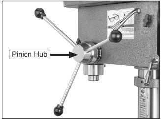
Figure 13. Downfeed handles installed.
