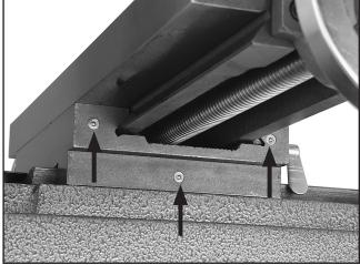
Figure 47. Oil fittings on left-side of table.
