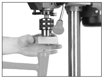
Figure 28. Seating the chuck on the arbor.
