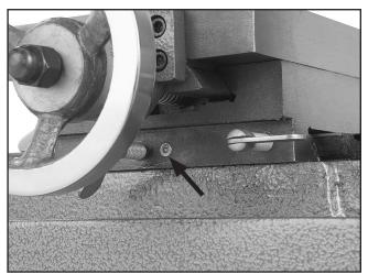
Figure 48. Oil fittings on right-side of table.
