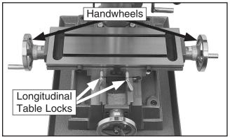
Figure 17. Longitudinal feed controls.
