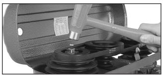
Figure 27. Tapping drawbar with hammer.
