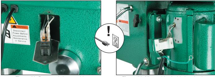
Figure 50. Power switch assembly.
