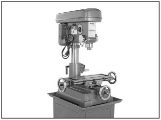
Figure 10. Headstock installed on base column.
