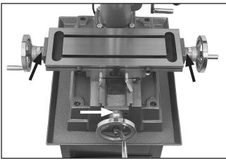
Figure 46. Handwheel oil fittings.
