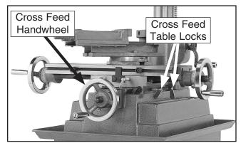
Figure 18. Cross feed controls.
