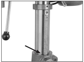
Figure 45. Rack & pinion greasing location.
