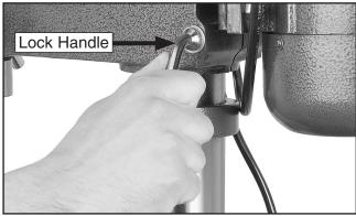
Figure 11. Securing headstock to column.
