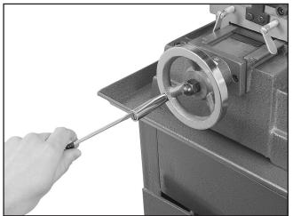
**Figure 12.** Installing handwheel handles. Model G0517 Mill/Drill
