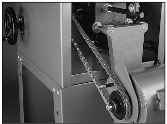
Figure 37. G3640 Power Twist® V-Belt installed.
