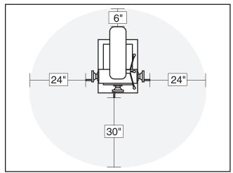
Figure 4. Overhead view of minimum working clearances.
