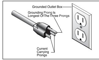
Figure 1. Typical 5-15 plug and receptacle.
