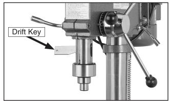
Figure 22. Drift key inserted in quill slot.
