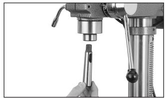
Figure 19. Installing a morse taper sleeve.
