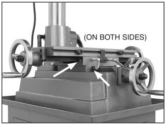
Figure 44. Cross feed and longitudinal ways.
