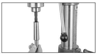
Figure 24. Inserting tooling into spindle.
