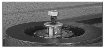
Figure 26. Nut unthreaded to top of drawbar.
