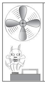
A CAUTION Many of the solvents commonly used to clean machinery can be toxic when inhaled or ingested. Lack of ventilation while using these solvents could cause serious personal health risks or fire. Take precautions from this hazard by only using cleaning solvents in a well ventilated area.
