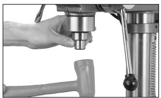
Figure 20. Tapping the sleeve into the spindle.
