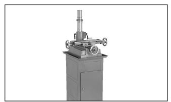
Figure 9. Base assembly attached to stand.
