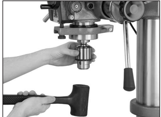
Figure 15. Seating arbor and drill chuck into the spindle.
