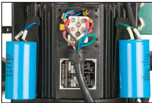
Figure 56. Spindle motor wiring.
