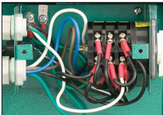
Figure 57. Spindle ON/OFF switch wiring.
